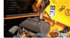
Frame Mounted Muffler (HSL850-7A)
