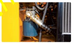
Remote Engine Oil Filter (HSL850-7A)
