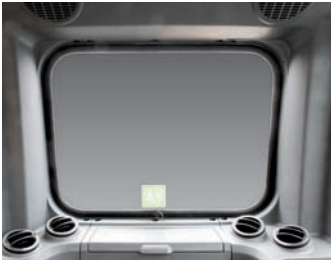
Rear Window Emergency Exit
