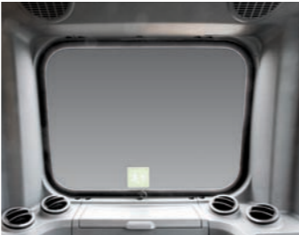
Rear Window Emergency Exit
