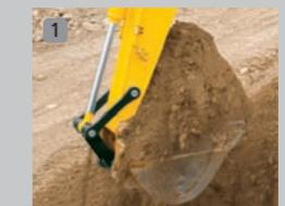
1 Reinforced Bucket and Bucket Linkage
