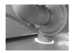
25. Fit the longer of the two rubber trim pieces (1440176H1) around the top edge of the hole with the flap toward the inside. If the machine has a hood-side, the shorter trim piece (1251075H1) fits around the bottom edge.
