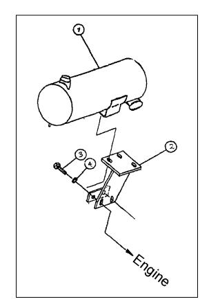
Installation of New Bracket and Muffler:
