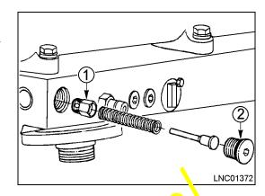
pressure for the filter by-pass valve. Plug (2) has a modified by-pass spring pocket. The pocket in the plug, where the spring is inserted, has been reduced by 3.65 mm (0.144 in.).
