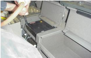
5- Disconnect wires to the timer-relay and remove the two screws to replace the timer-relay
