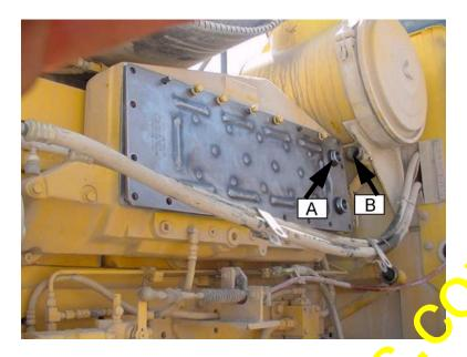
Install the aftercooler using the guide pins to support the weight of the assembly. The O-Rings that are used to seal the elbows from the aftercooler to the elbow (Arrow A) and the elbow to the transfer tube (Arrow B) should be lubed with Lithium grease. Lithium grease will allow the parts to slide over each other without damaging the O-Rings.
