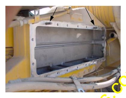
Before removing the aftercooler cut two 3/8 in. screws with 1 in. of shan exposed as shown by the arrows above. These screws will serve as guides when removing and installing the aftercooler. Clean the aftercooler housing surface where the new aftercooler will be installed.
