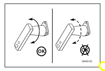
**NOTE:** The Permaglide Teflon<sup>TM</sup> bushing works by transferring a Te Ton<sup>TM</sup> coating to the shaft during operation. The Teflon<sup>TM</sup> coating on the shaft should **not** be removed except for cleaning rust and debris from the shaft, in which case the bushings should be replaced.
