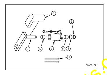
Use an arbor press to install the new bushings (5) into the pivot sneet support (6).
