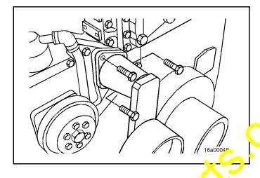
Remove the three mounting capscrews that are holding the pivor sport to the idler pulley bracket.
