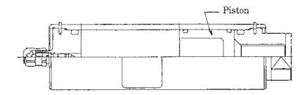
(1) The number of O-rings used for the piston has been changed from 1 to 2.
