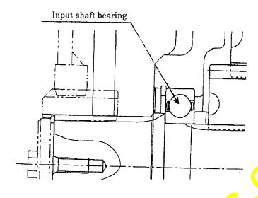
The input shaft bearing illustrated above have been improved
