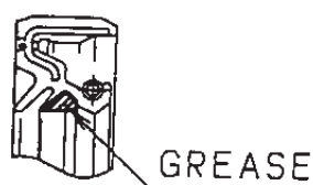
The space to fill grease
