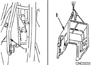
9. Remove the complete Donaldson air cleaner assembly, aspirator system and mounting brackets shown in the illustration below.
