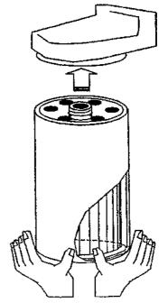
③ After fully filling the filter vith the fuel, remove the cap (N and discard the removed va
