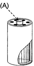
② With the cap (A) installed, pour the fuel into the filter.
